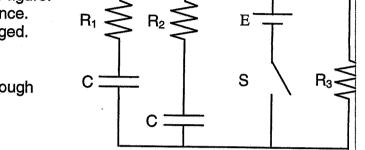
10. Just after the switch is closed, what is the current through resistor R<sub>3</sub>?
