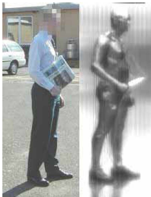
Fig. 5. (Color online) 94 GHz radiometer image taken outdoors with cold sky illumination (courtesy of R. Appleby).
