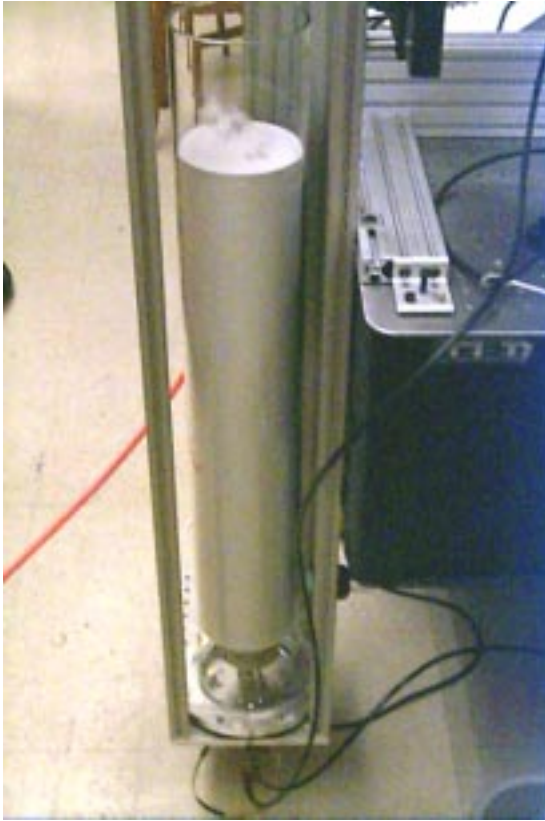
Fig 3b Fluidized Bed of Sand
