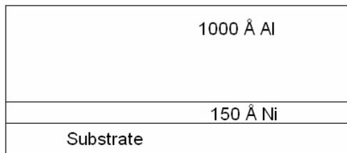
Figure 2 – Diagram describing sample structures - a thin nickel layer for silicide formation is followed by a thicker layer of aluminum, for electrical contact
