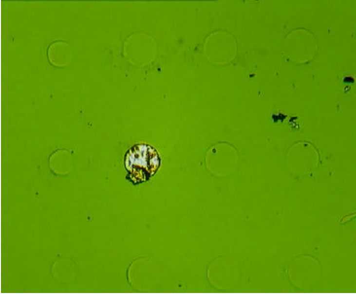
Figure 8 – Destruction of samples with a Mo barrier layer during mesa etch
