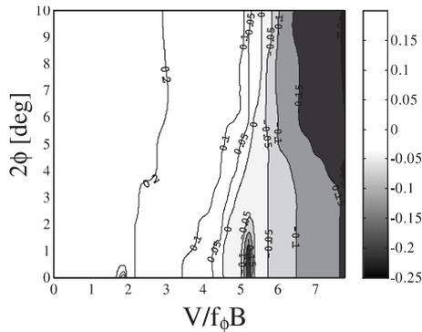
Fig. 4. Velocity–amplitude–damping diagram.
