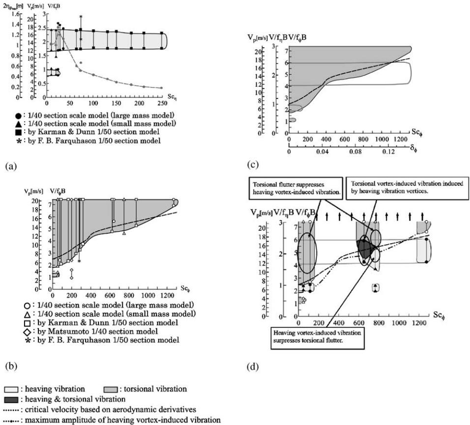
Fig. 7. Effects of Scruton number on aerodynamic interferences: (a) heaving 1DOF, (b) torsional 1DOF, (c) heaving 1DOF + torsional 1DOF and (d) 2DOF.
