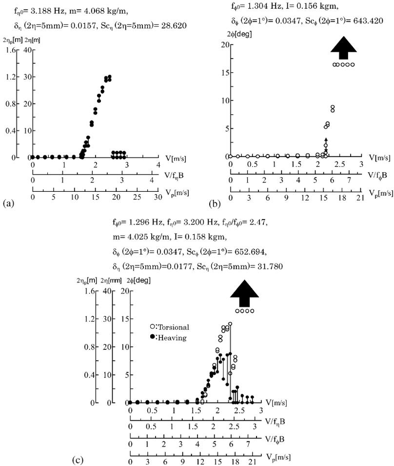
Fig. 5. Velocity–amplitude diagrams: (a) heaving 1DOF, (b) torsional 1DOF and (c) 2DOF.
