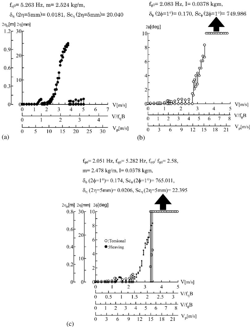
Fig. 3. Velocity–amplitude diagrams: (a) heaving 1DOF, (b) torsional 1DOF and (c) 2DOF.
