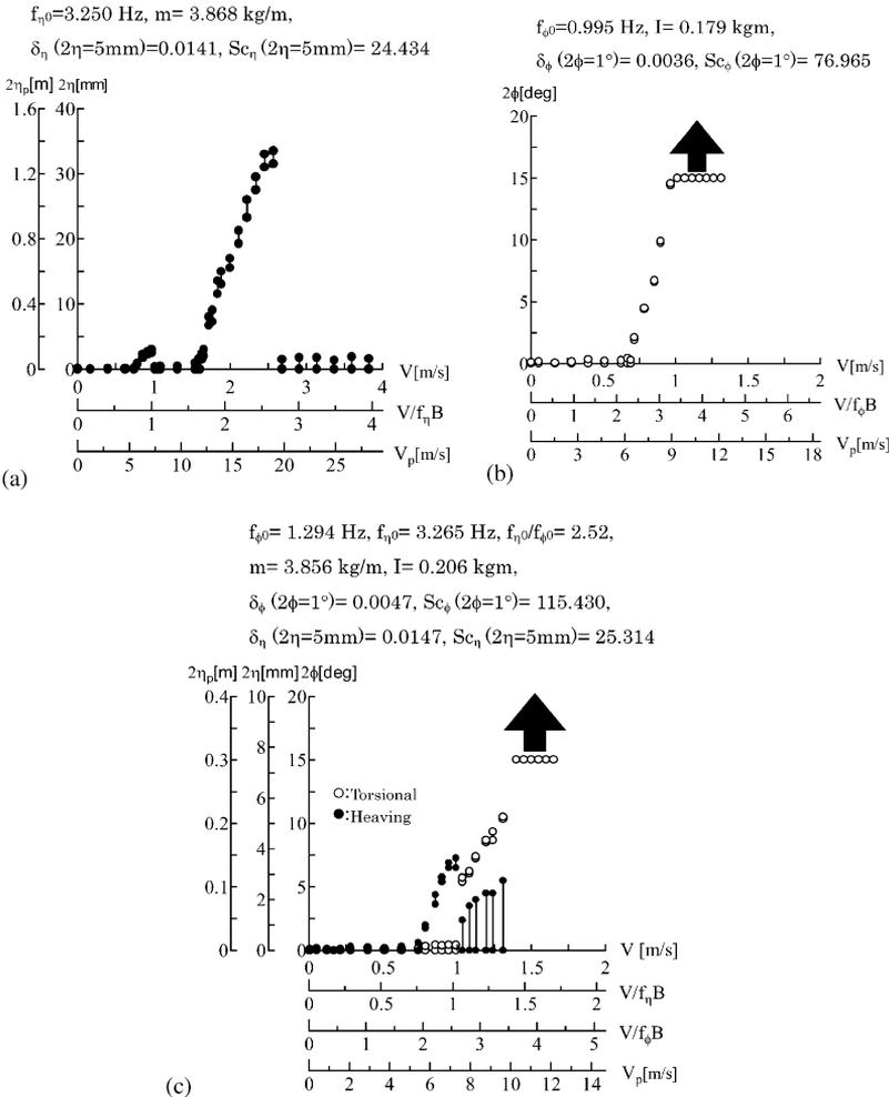
Fig. 2. Velocity–amplitude diagrams: (a) heaving 1DOF, (b) torsional 1DOF and (c) 2DOF.
