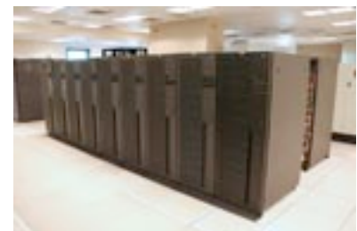
The IBM Mass Storage System at the Ohio Supercomputer Center will receive and store data from the Large Hadron Collider's ALICE experiments in Switzerland. (Photo © OSC)
