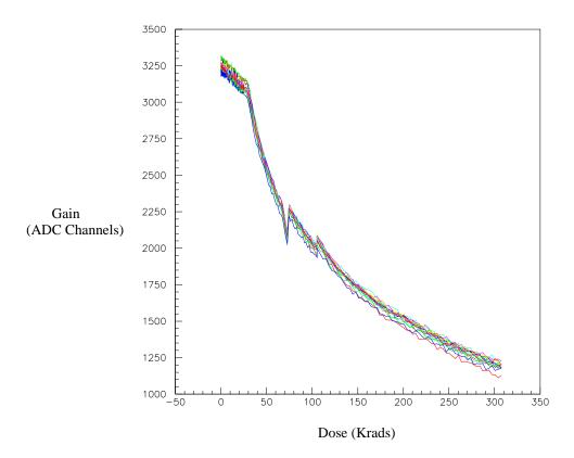
The plot above shows the gain of the 16 buckeye channels as a function of radiation dose. Five separate runs with different beam intensity make up this plot. The lower the beam intensity the less effect the radiation has on the chip gain. One can also see annealing recovery of the chip between runs. We expect less than 10 KRads during 10 years of LHC running. Thus the buckeye chip behaves well in radiation.
