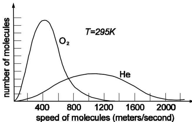
Because the shape of these graphs is known, the average kinetic energy of a molecule of the gas can be calculated and is found to be directly proportional to the absolute temperature of the gas. Recall that kinetic energy can be expressed as
