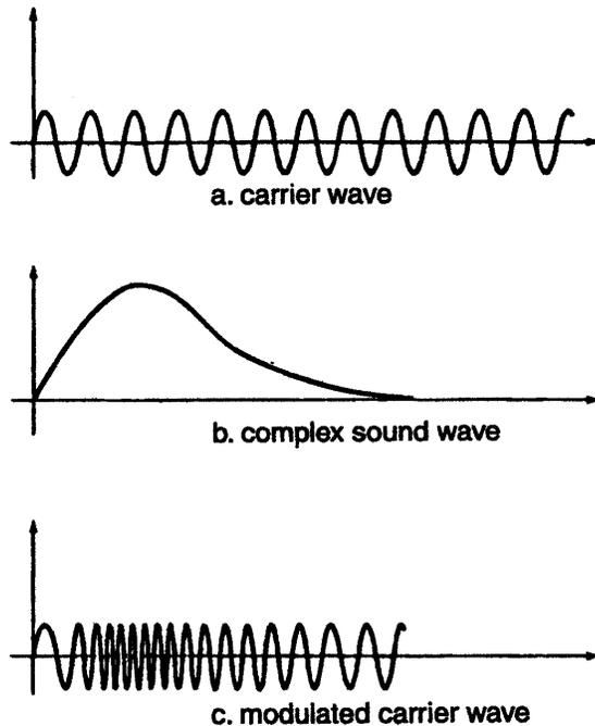
Because FM radio works on the principle of frequency modulation, the actual frequency of the transmission will vary. Therefore, instead of broadcasting at a single frequency, FM radio broadcasts over a range of frequencies. The range of frequencies over this bandwidth is small compared to the frequency of the FM carrier wave. This means that the FM station can still be assigned a single frequency.
