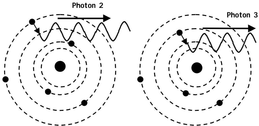
**Time 3: The electron drops down one energy level and emits one photon of visible light.**
