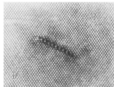
Transition electron microscope picture of the extended silicon interstitials.
