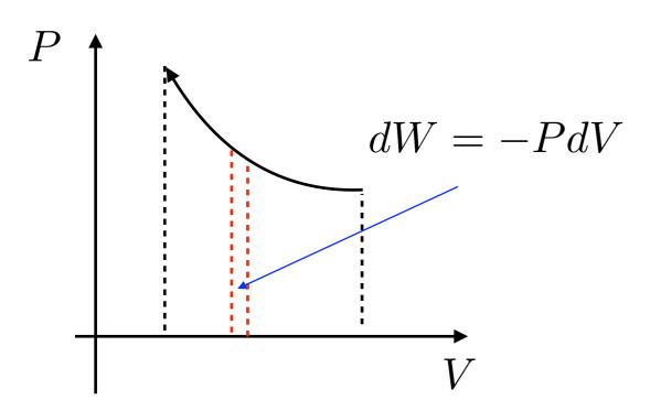
Gas is pushed in, work is done ON the gas
