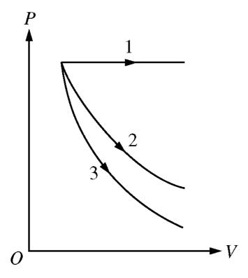
29. For an ideal gas, consider the three thermodynamic processes—labeled 1, 2, and 3—shown in the *PV* diagram above. Each process has the same initial state and the same final volume. One process is adiabatic, one is isobaric, and one is isothermal. Which of the following correctly identifies the three processes?
