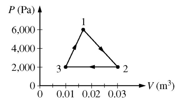
28. A sample of nitrogen gas undergoes the cyclic thermodynamic process shown above. Which of the following gives the net heat transferred to the system in one complete cycle  $1 \rightarrow 2 \rightarrow 3 \rightarrow 1$ ?
