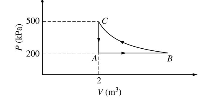
37. A constant amount of an ideal gas undergoes the cyclic process *ABCA* in the *PV* diagram shown above. The path *BC* is isothermal. The work done by the gas during one complete cycle, beginning and ending at *A*, is most nearly
