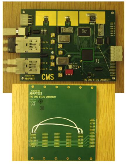
With Virtex2 Pro FPGA (XC2VP2-5FG456): DMB to FPGA
