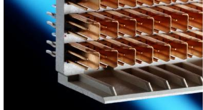
VME P3 spaces, 6.4 Gbps rated connector Data from DDU to DCC TTC control bus (clock, L1A, command/data)
