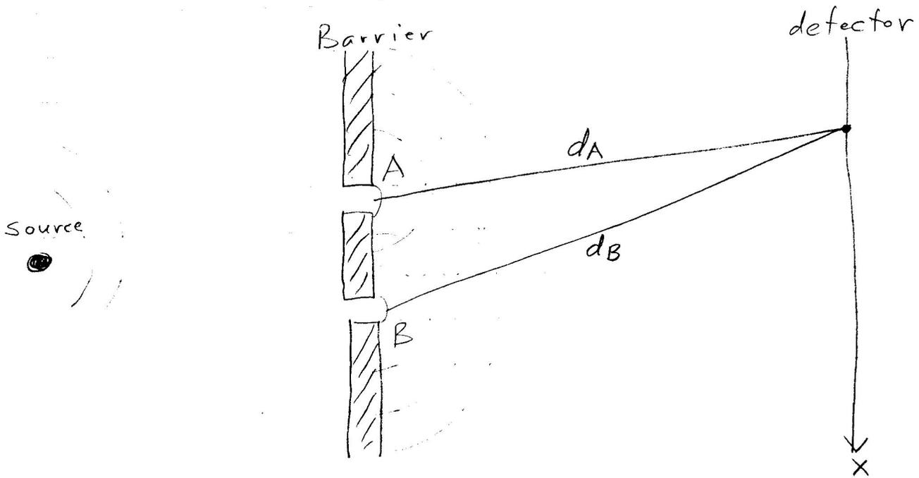
Slits A and B act as secondary sources for wave at detector
